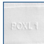
PROflo<sup>+</sup> filter bag series are embossed with the filter media and micron rating to allow for quick and easy product identification. Traditional paper tags are either removed or destroyed in filtration applications which can lead to misidentification and result in costly production errors. By heat embossing the felt surface, a permanent marking on the filter is created which helps to ensure easy identification and reduce the probability of production errors.
